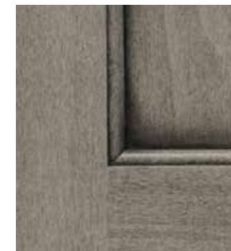
Aggressive Sand-through Shown on stained finish
