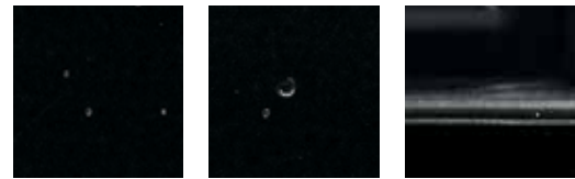
Wormholes Dents Wear Shown on painted finish
