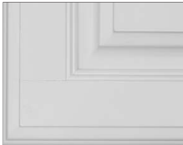
Example of front joint separation
